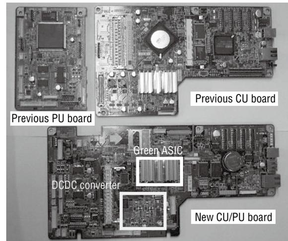
**Figure 5. Comparison of Control Boards**
