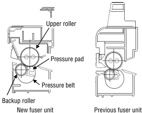
**Figure 3. Fuser Unit Cross Sections**
