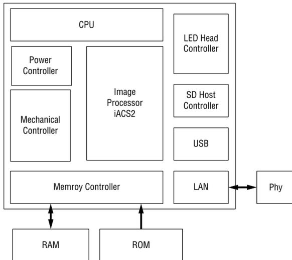
Figure 4. Block Diagram of Green ASIC
