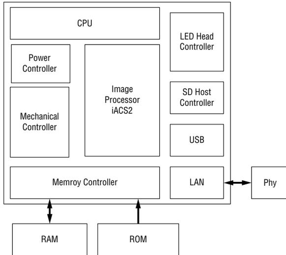
**Figure 4. Block Diagram of Green ASIC**
