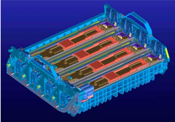
Figure 2. Integrated Image Drum Unit
