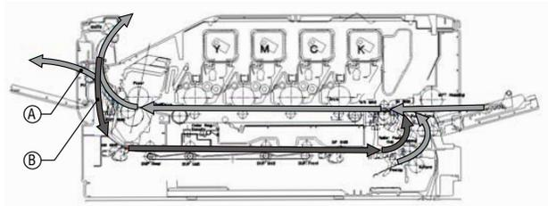
Figure 1. Printer Cross-section and Paper Path
