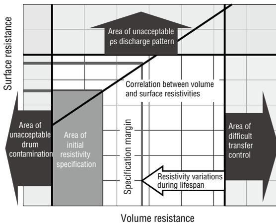
**Figure 7. Favorable Range of Transfer Belt's Volume and Surface Resistivities**
