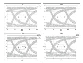
Figure 4. Eye Pattern of High-speed Long Transmission FPC
