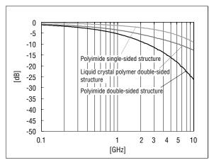
Figure 3. Insertion Loss (IL) of Highspeed Long Transmission FPC
