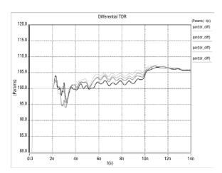
Figure 2. Impedance of High-speed Long Transmission FPC (100Ω Differential)
