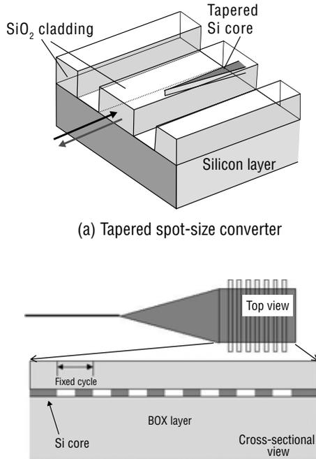
Figure 9. Couplers for Different Optical Elements
