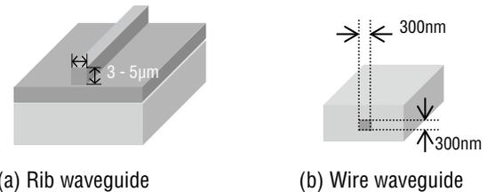
Figure 1. Waveguide Structures
