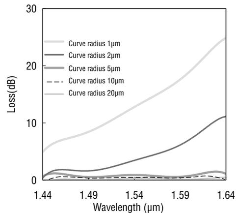
Figure 5. Loss Measurements for Curved Waveguides
