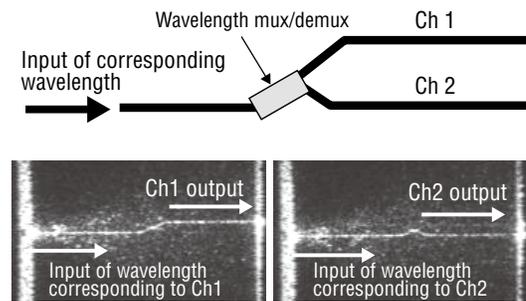
Figure 8. Observed Light Trajectories of Wavelength Mux/Demux
