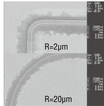
Figure 4. SEM Images of Curved Waveguides for  $R=2$  and  $20\mu\text{m}$
