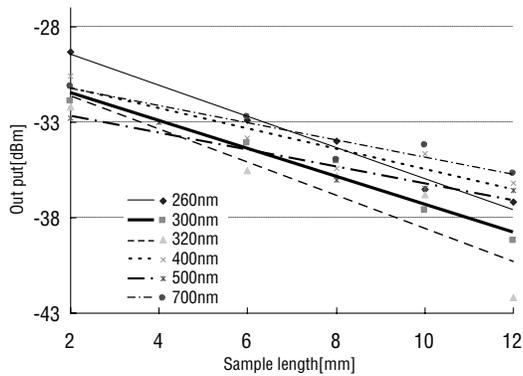
Figure 3. Straight Waveguide Propagation Losses
