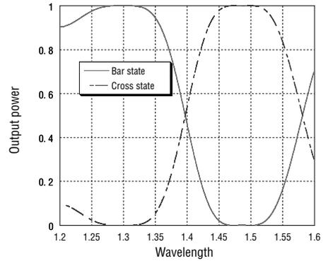
Figure 7. Four-stage Mach-Zehnder Wavelength Mux/Demux Two-dimensional FDTD Simulation Results
