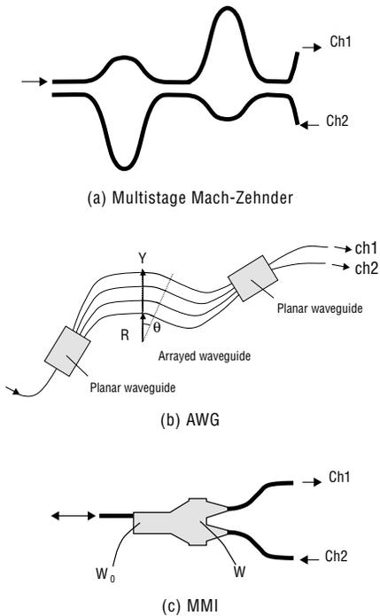
Figure 6. Overview of Wavelength Mux/Demux
