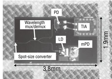
Figure 10. Sample of a Bi-directional Communication Module
