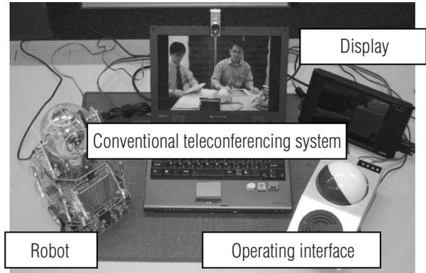
Fig. 2 System configuration diagram
