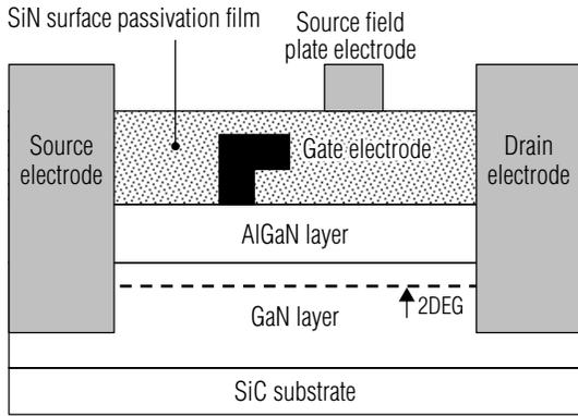
**Fig. 2 Schematic cross-section of GaN-HEMT**
