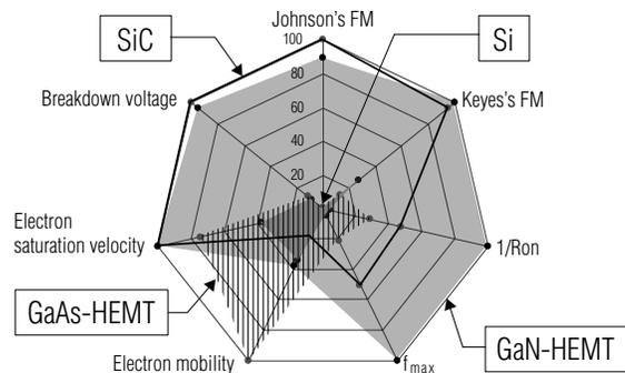
**Fig. 1** Diagram with performance indices and materials of respective devices
