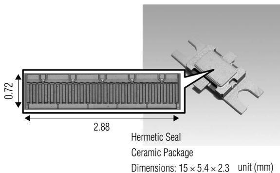
**Photo 1** Microphotograph of 50 W-class GaN-HEMT with multi-finger gate and mounted ceramic package
