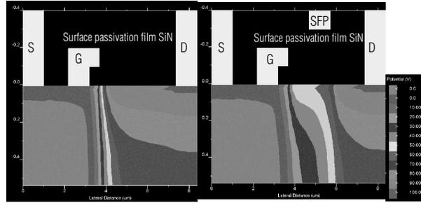
**Fig. 4 Relaxation effect of electrical potential distribution using SFP electrode**
