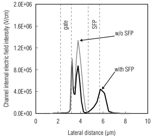
**Fig. 5 Change of electric field intensity in channel using SFP electrode**
