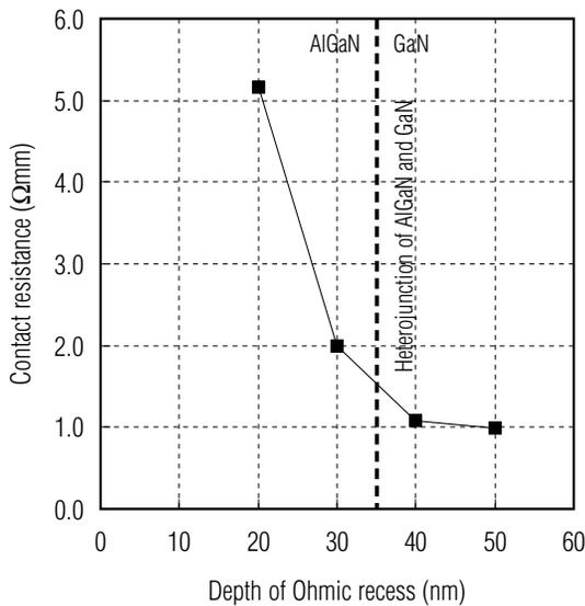
**Fig. 3 Dependence of contact resistance on recess depth in ohmic region**
