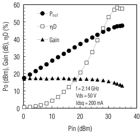
**Fig. 8** Input and output power characteristics of recently developed 50 W-class GaN-HEMT
