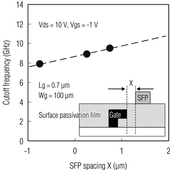
**Fig. 6 SFP position influence on cut-off frequency**
