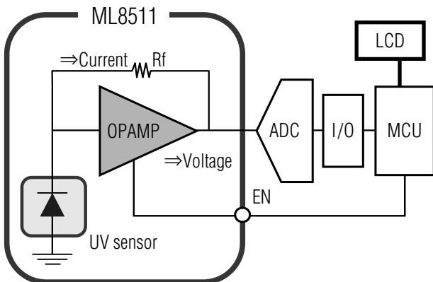
Fig. 2 Example of configuration for UV meter using ML8511
