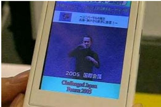
**Fig. 6** Display of sign language image on handheld device
