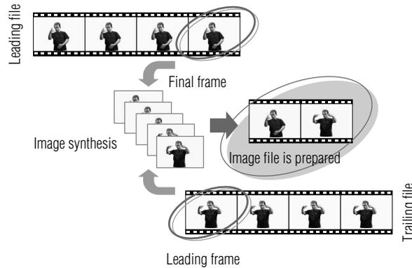
**Fig. 4 Flow of image synthesis**
