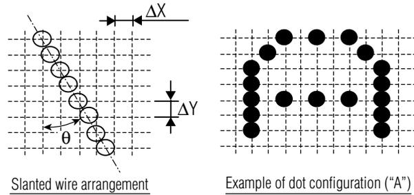
Fig. 5 Simulated wire arrangement diagram
