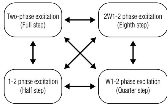
**Fig. 6 Switching of excitation methods while motor is turning**
