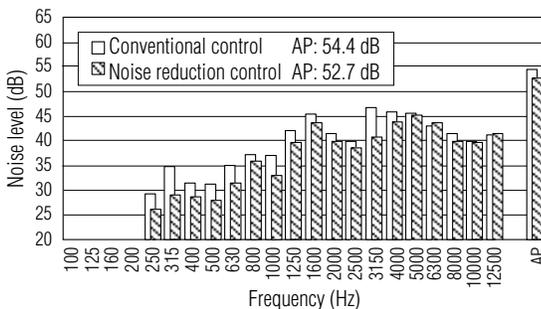
Fig. 9 Noise level for driving in all ranges
