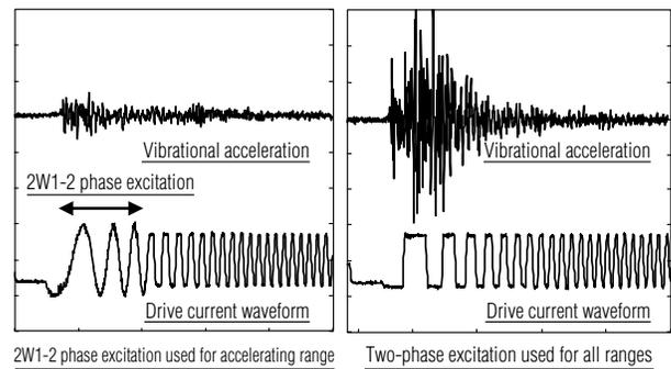
**Fig. 7 Frame vibration acceleration temporal waveform during spacing operations**
