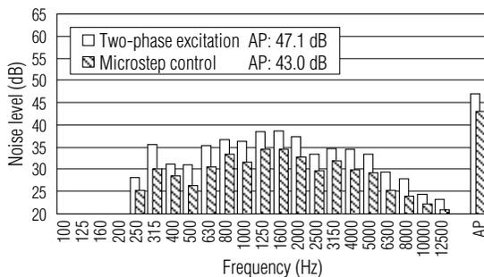
Fig. 8 Noise level when motor is driven only for spacing operation
