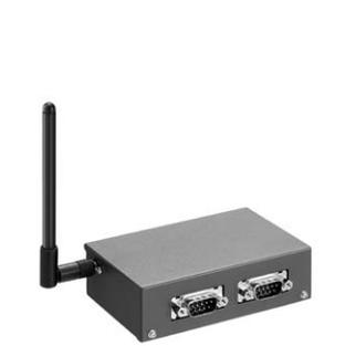
**Photo 2 ZigBee wireless marker**
