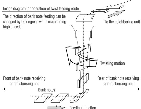
Fig. 5 Image diagram of twist feeding
