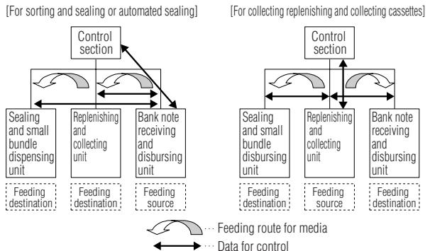
**Fig. 6 Equipment internal control mode**
