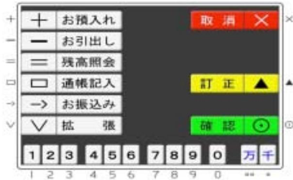
Fig. 3 Example of tactile symbols screen
