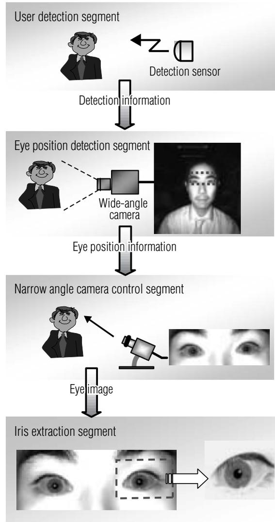
Fig. 2 Fully automated iris image capturing segment
