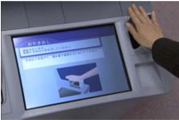
**Photo 2** Image of authentication using palm vein sensor
