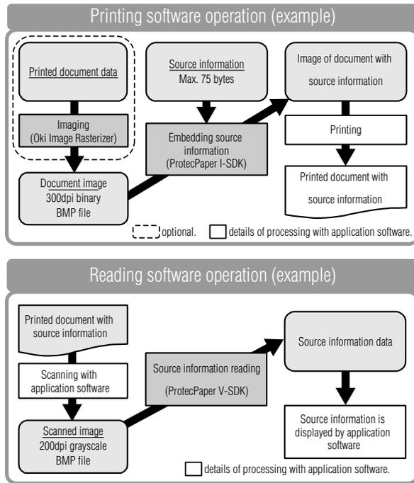
Fig. 3 Example of software operation using ProtecPaper SDK
