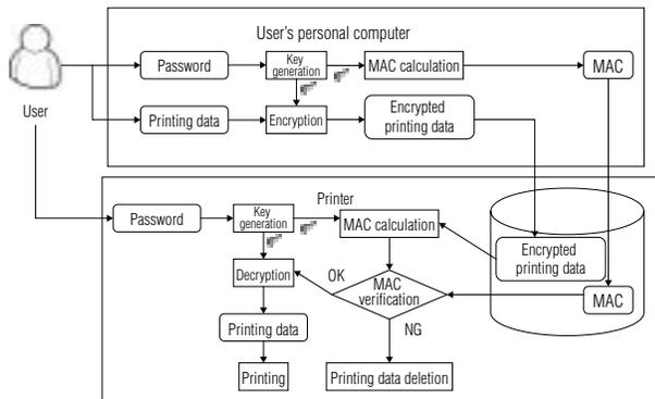
**Fig. 2 Process for encrypted authenticated printing**
