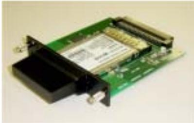
Photo 1 Overview of built-in wireless LAN board
