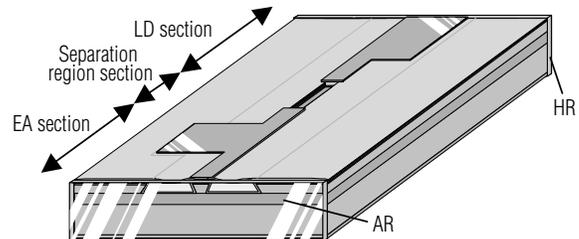
Fig. 1 Schematic structure of EMwL chip
