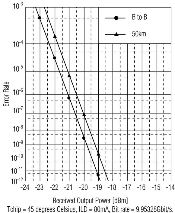
Fig. 8 Bit error rate characteristics
