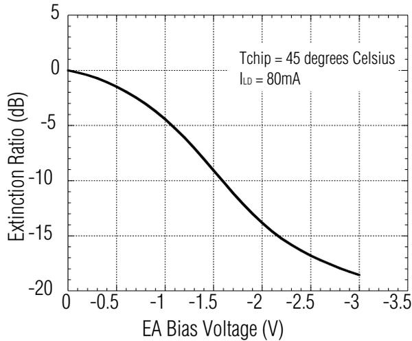
Fig. 5 Optical extinction characteristics
