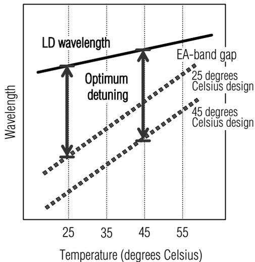
Fig. 2 Schematic diagram of temperature dependency of detuning
