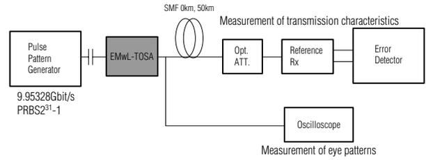
Fig. 6 Transmission characteristics evaluation system
