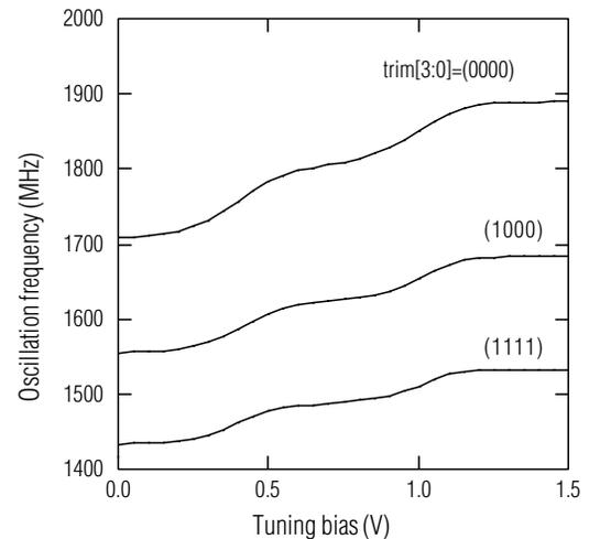
**Fig. 4 Oscillation frequency of voltage-controlled oscillator**
