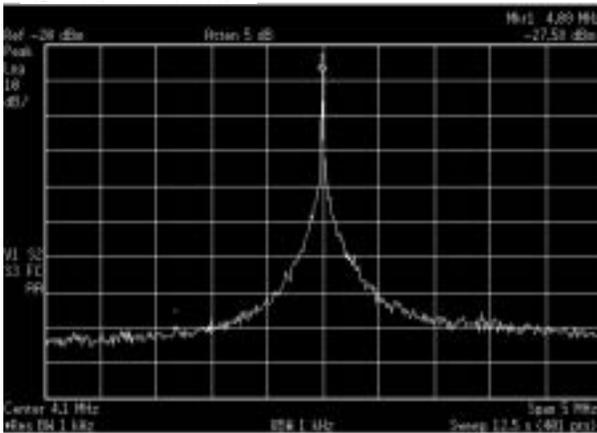
**Fig. 5 Spectrum of intermediate frequency with phase-locked loop**
