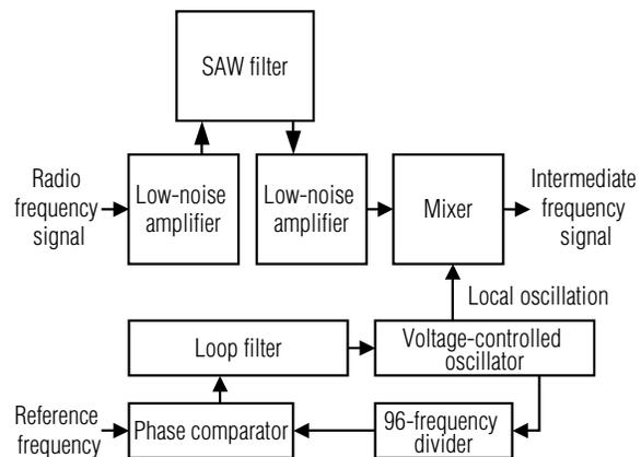
**Fig. 3 Global positioning system receiver developed using the SOS technology (The figure only shows the radio frequency segment of the circuit.)**
