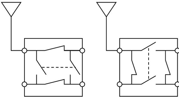
**Fig. 2 Switching action of double-pole double-throw antenna switch**
