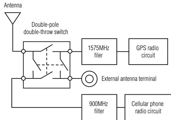
Fig. 1 An example of usage of antenna switch
