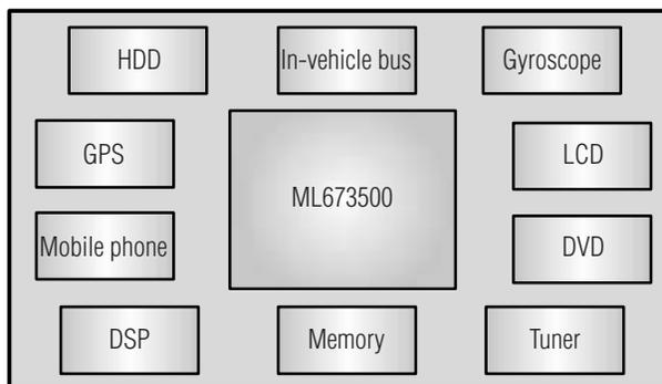
**Fig. 1** An example of an application for audio visual navigation and communication integrated system.
