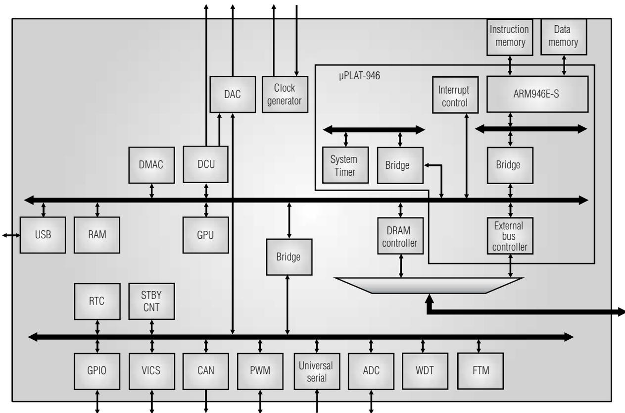
**Fig. 2 Configuration diagram of the ML673500**
