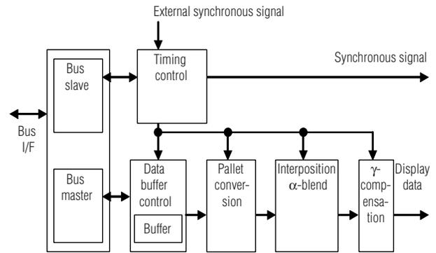
Fig. 2 Block diagram of display controller
