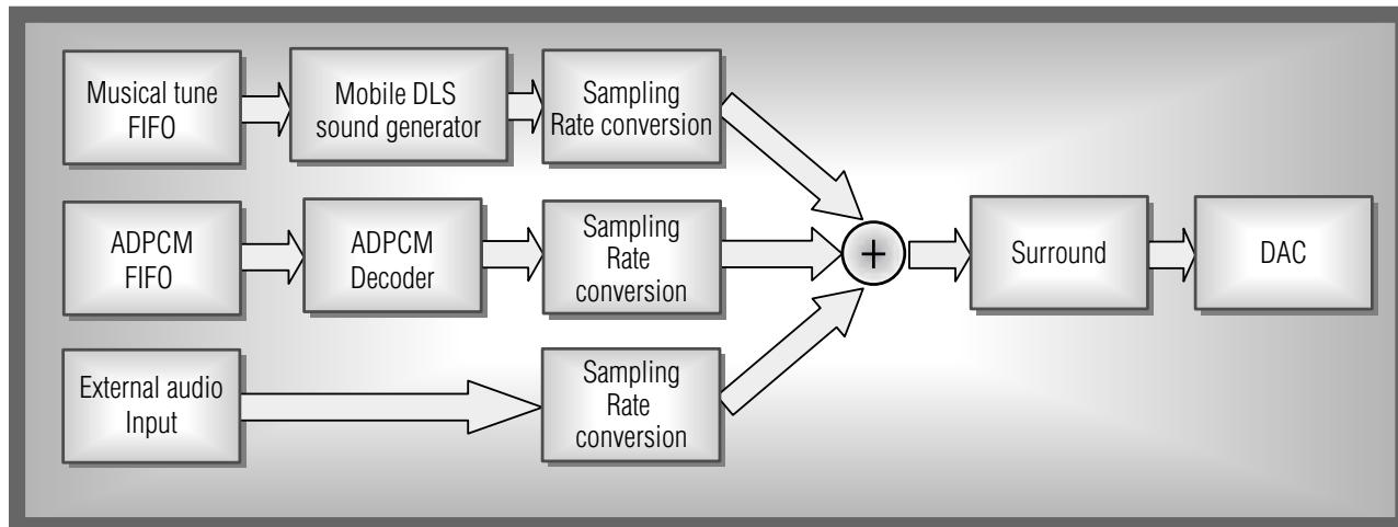
Fig. 1 MD-64RM function configuration diagram
