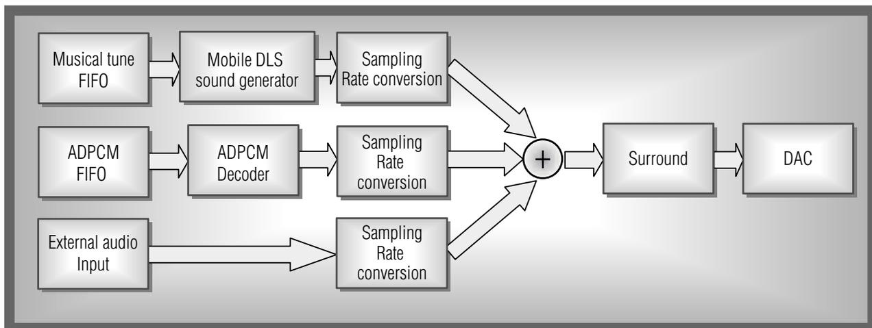
Fig. 1 MD-64RM function configuration diagram
