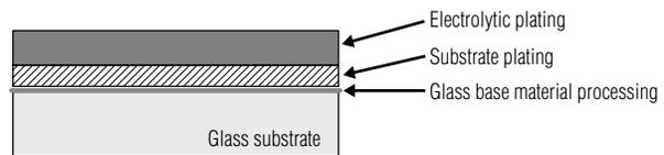
**Fig. 2 Description of an evaluation glass substrate structure.**
