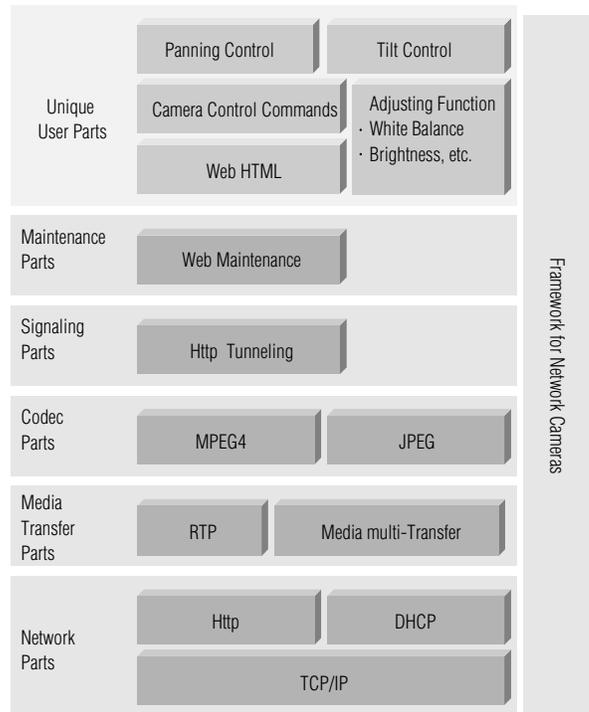
Fig. 4 Network camera platform
