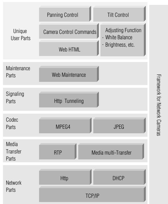
Fig. 4 Network camera platform
