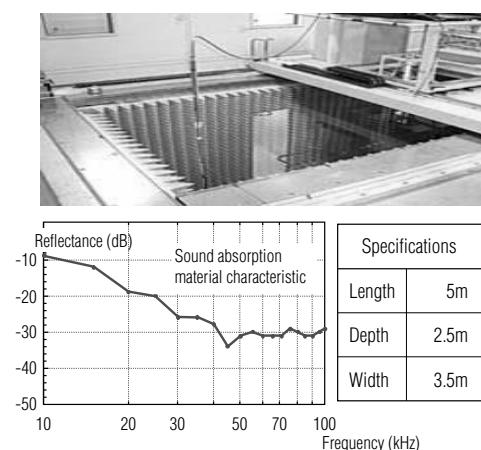
Fig. 4 Anechoic water tank.
