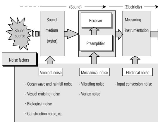
Fig. 1 Noise factors relating to hydroacoustic measurements.
