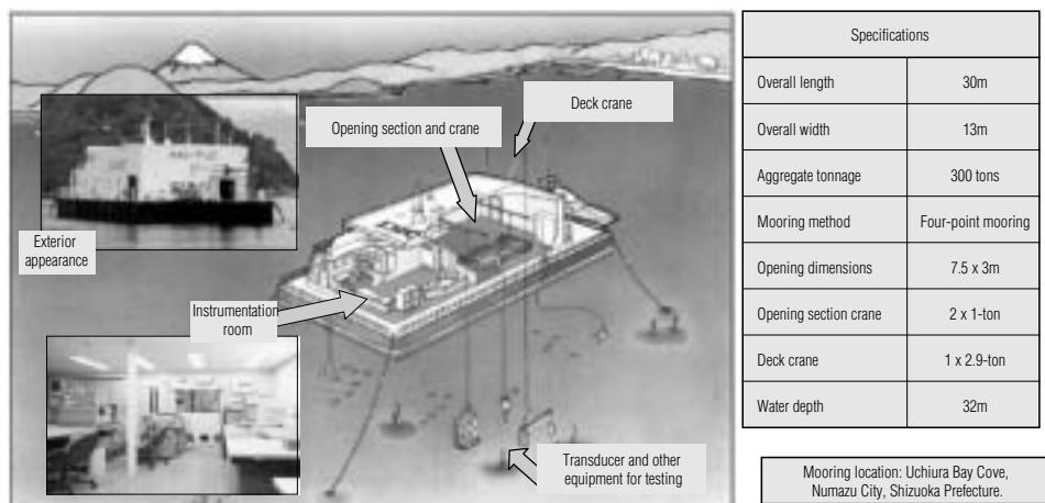
Fig. 2 Marine instrumentation barge (Seatec II).
