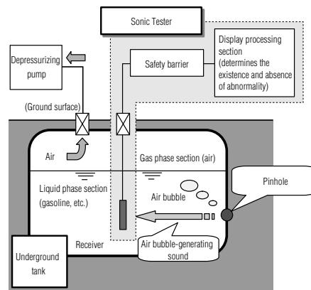
Fig. 9 Summary of an inspection with a Sonic Tester.
