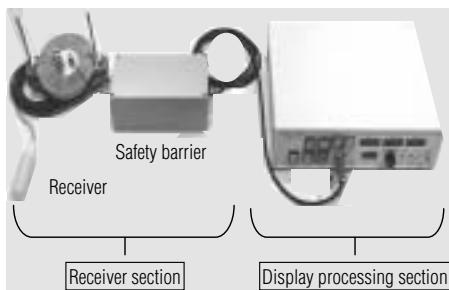
Fig. 8 Configuration of a Sonic Tester.
