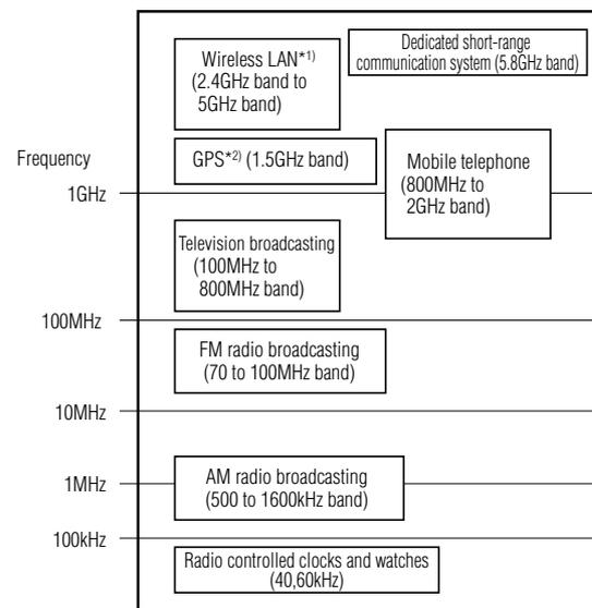
Fig. 1 Radio frequencies for wireless equipments
