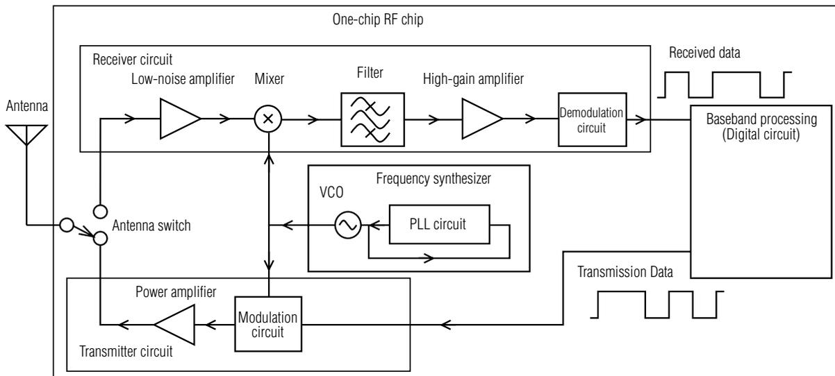
Fig. 2 Configuration example of RF circuit
