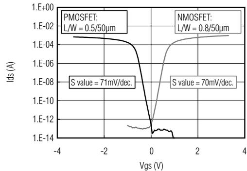
Fig. 8  $I_{ds} - V_{gs}$  characteristics of an SOS MOSFET with a gate length of 0.5µm
