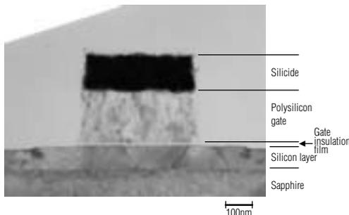
**Fig. 4 Transmission electron microscopic photograph of a cross section of an SOS MOSFET device**
