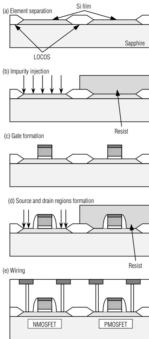
Fig. 7 Fabricating process flow of an SOS device
