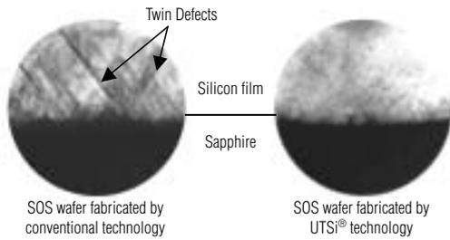
**Fig. 3 Transmission electron microscopic photograph<sup>9)</sup> of a cross section of an SOS wafer**
