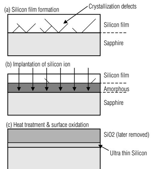
**Fig. 2 SOS wafer fabricating flow**
