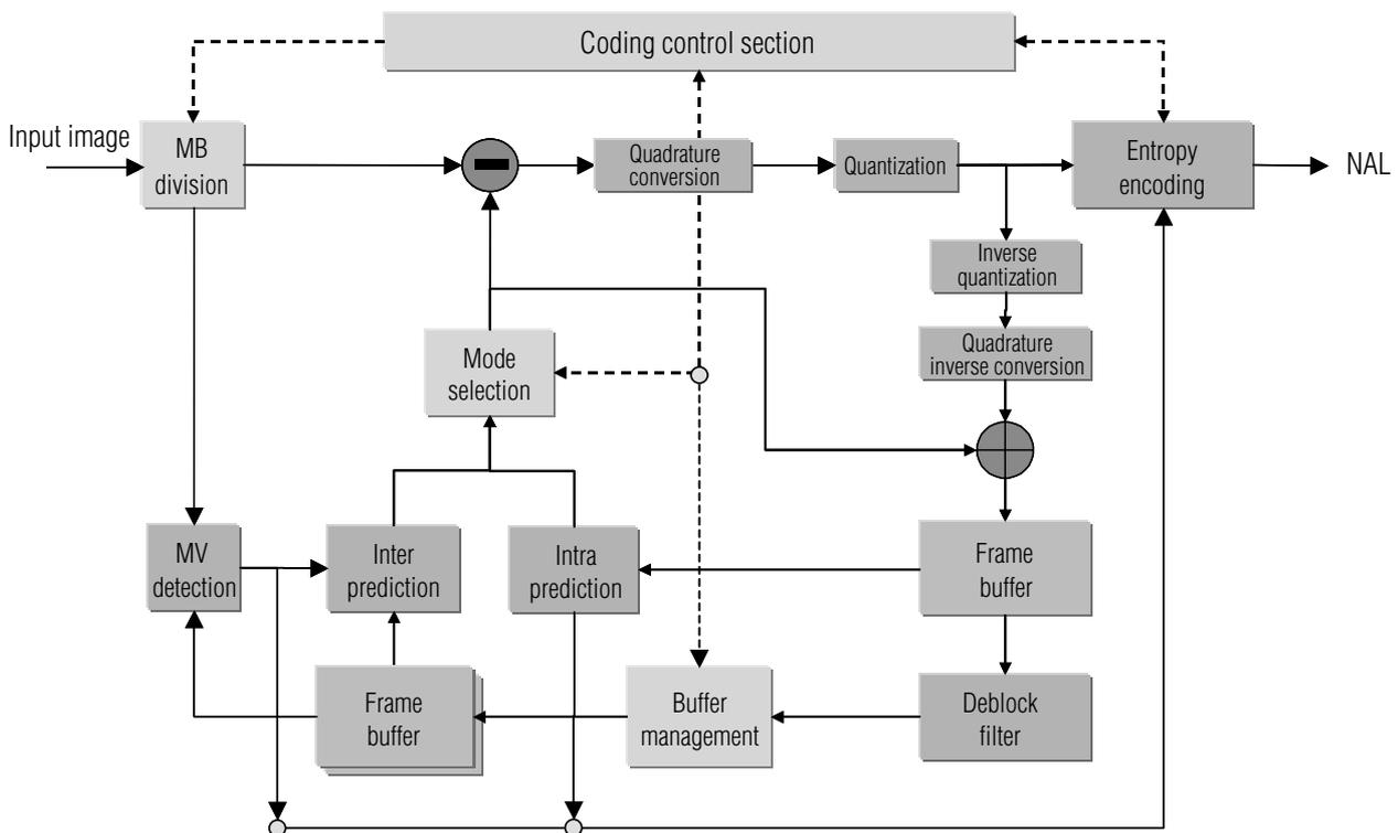
Fig. 1 Composition diagram of MPEG4-AVC/H.264
