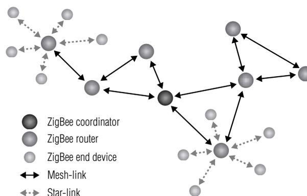
**Fig. 2 Network model of ZigBee**
