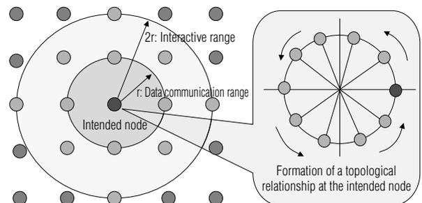
Fig. 4 Network model of ZigBee
