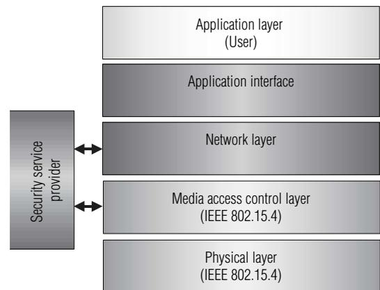
Fig. 1 Protocol structure of ZigBee
