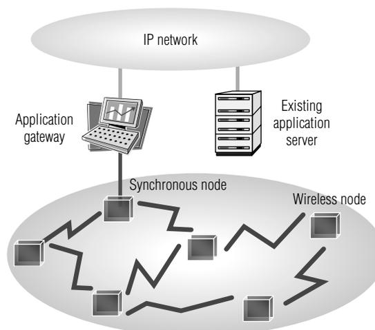
Fig. 5 Configuration of the platform for the feasibility test
