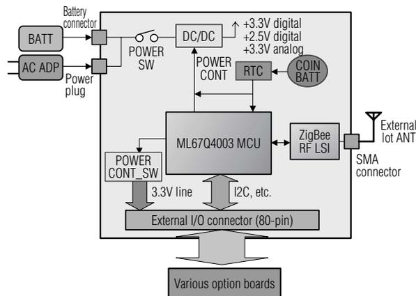
Fig. 6 External view (upper) and configuration diagram (lower) of the wireless node for feasibility experiments
