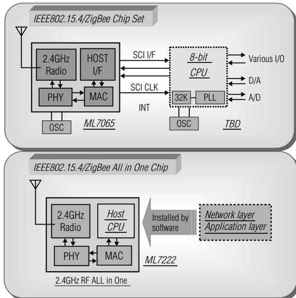
Fig. 3 The complete IEEE 802.15.4 compliant wireless LSI (above) and the ZigBee compliant one-chip wireless LSI (below).
