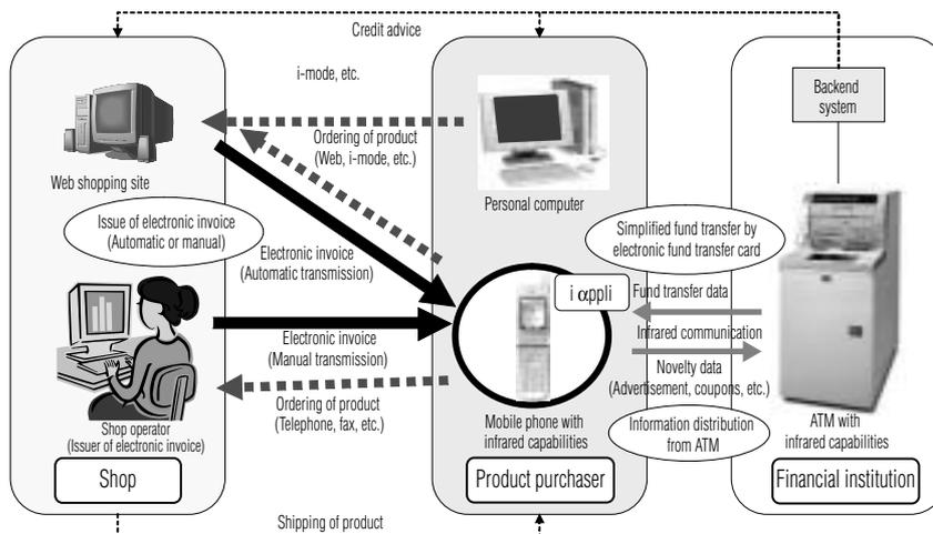
Fig. 3 Prototyped mobile electronic invoice system
