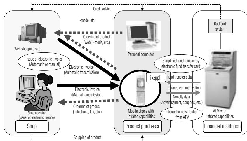
Fig. 3 Prototyped mobile electronic invoice system
