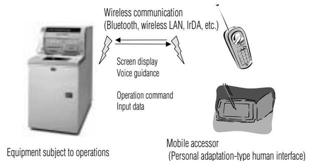
Fig. 1 Basic configuration and basic concept of mobile accessor
