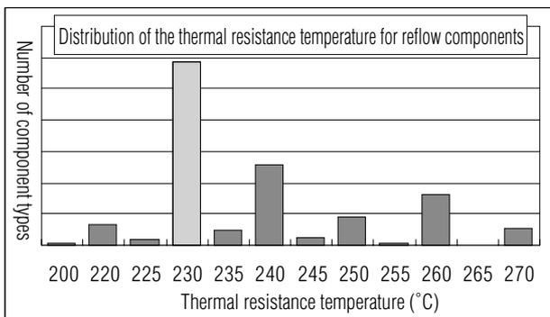
Fig. 2 Reflow thermal resistance temperature and number of component types
