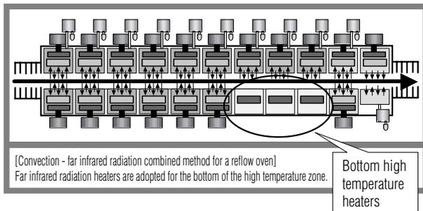
Fig. 5 Structure of a reflow oven (cross section diagram)
