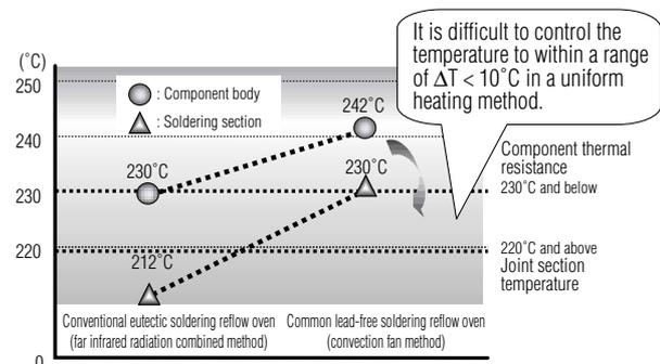
Fig. 4 Comparison of the temperature variance between substrates
