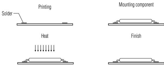
Fig. 1 Summary of reflow soldering
