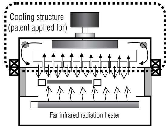
Fig. 6 Structure of a reflow oven (front view)
