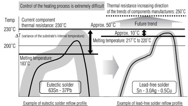
Fig. 3 Comparison of temperature margins of lead-free solder and eutectic solder
