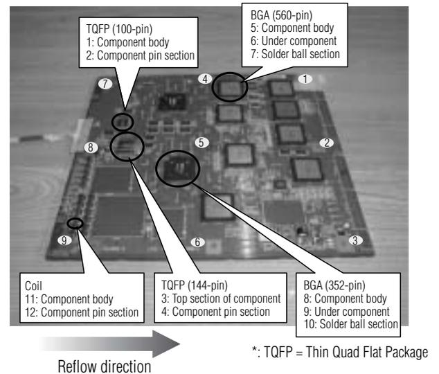
Fig. 7 Substrate used for the verification of effects and measurement locations
