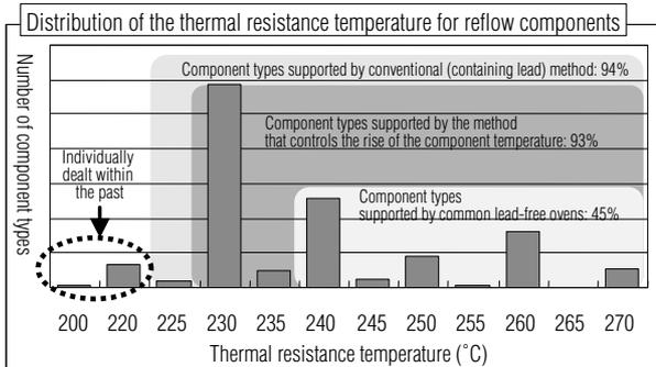
Fig. 9 Reflow thermal resistance temperature and number of component types (result after applying the temperature rise controlled method)
