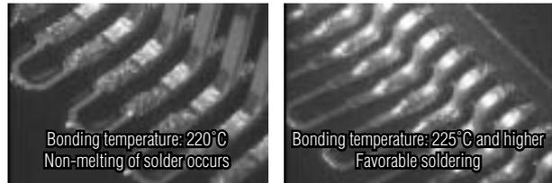
Photo 1 Reflow temperatures and conditions of soldering
