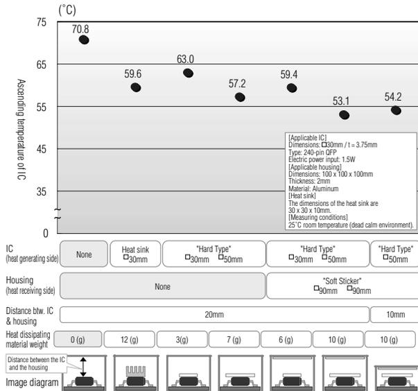
**Fig. 3 Heat dissipating characteristics of the Stick-it Flexible**
