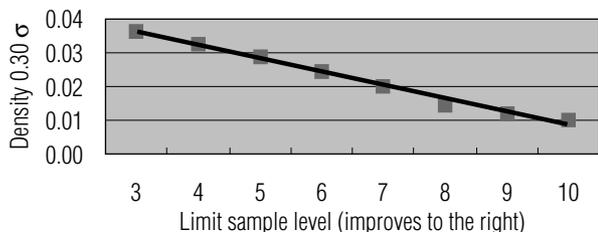
Fig. 12 Relationship between limit sample level and  $\sigma$
