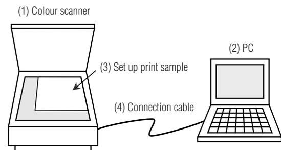
Fig. 1 Simple image evaluation system
