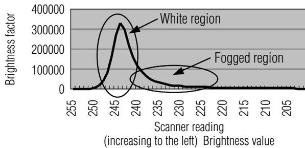
Fig. 6 Brightness distribution of fogging sample
