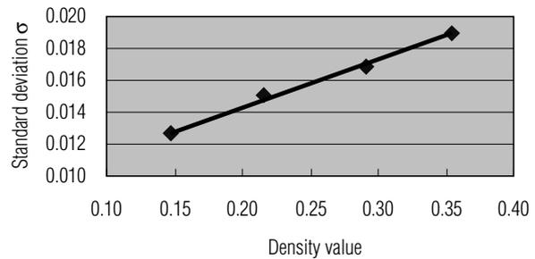
Fig. 11 Relationship between standard deviation  $\sigma$  and density
