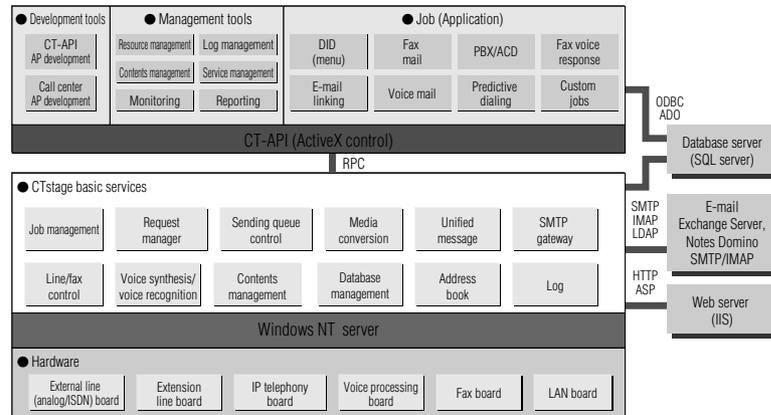
Fig. 3 CTstage software configuration
