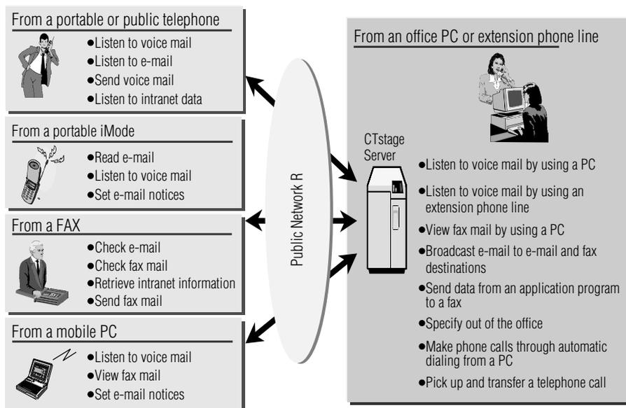
Fig. 2 Conceptual diagram of the unified messaging function
