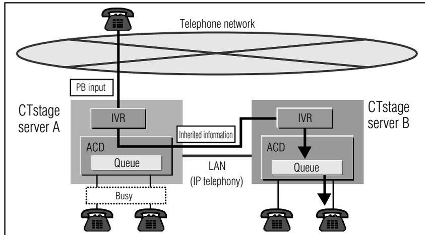
**Fig. 8 Conceptual diagram of a distributed call center**
