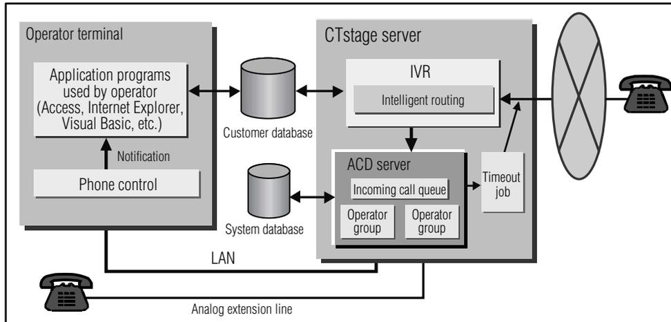
Fig. 6 Conceptual diagram of the call center system
