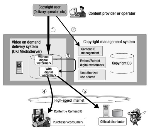
Fig. 1 Copyright management system and video delivery system2)
