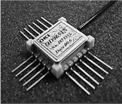
Fig. 8 External view of 10 Gb/s PIN-AMP module
