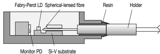
Fig. 5 Cross section of OL3312N
