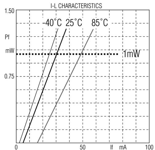
Fig. 6 Optical characteristics of OL3312N
