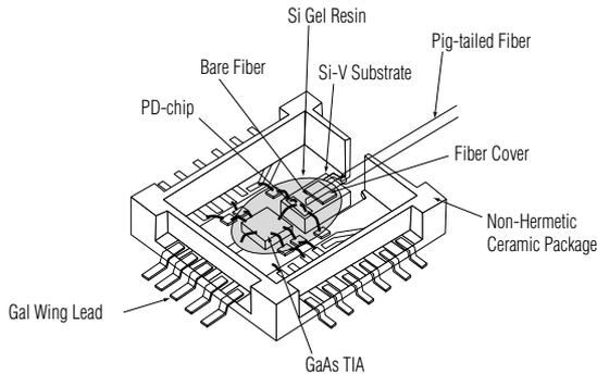
Fig. 9 Structure of 10 Gb/s PIN-AMP module
