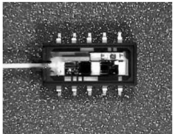
Fig. 2 Structural diagram and external view of ONU optical module for ATM-PON
