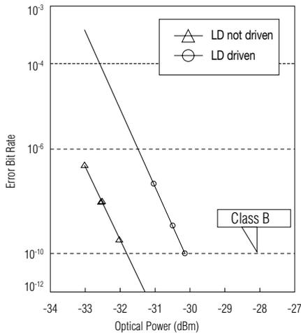
Fig. 3 Error rate measurement results (at 25 °C)
