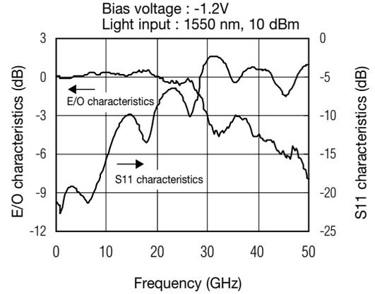
Fig. 6 Frequency characteristics
