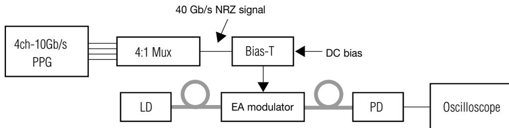
Fig. 8 Measurement system of 40 Gb/s signal modulation experiment
