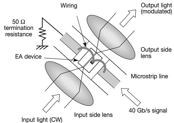
Fig. 3 Mounting structure for EA device
