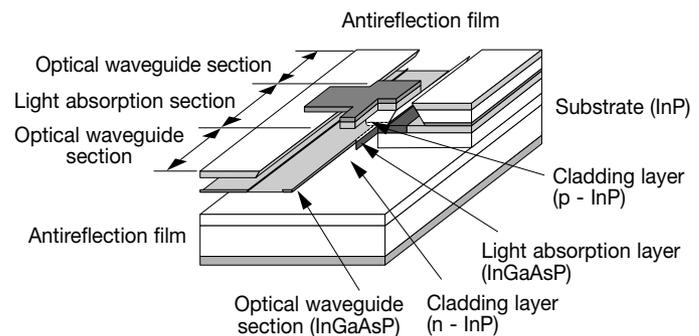
Fig. 4 Structure of EA device
