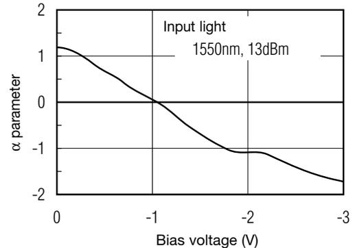
Fig. 7 Chirp characteristics
