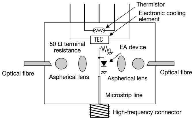
Fig. 2 Structure of EA modulator module
