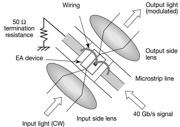
Fig. 3 Mounting structure for EA device
