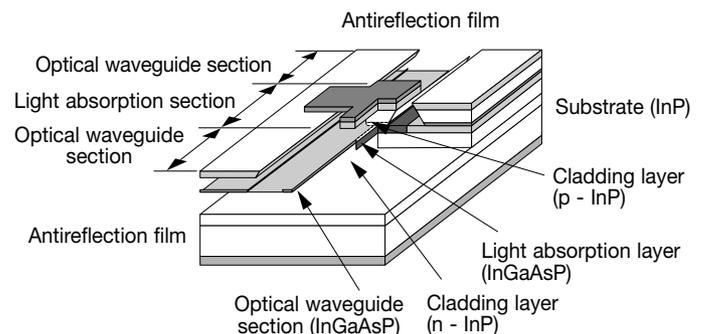
Fig. 4 Structure of EA device
