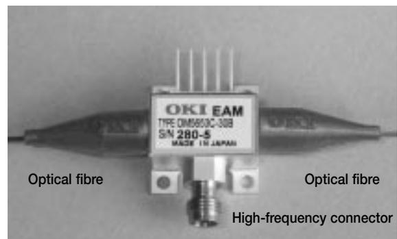
Fig. 1 External photograph of EA modulator module
