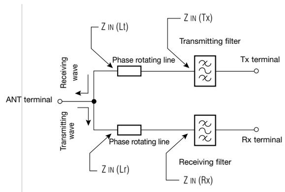
Fig. 9 Composition of SAW antenna duplexer
