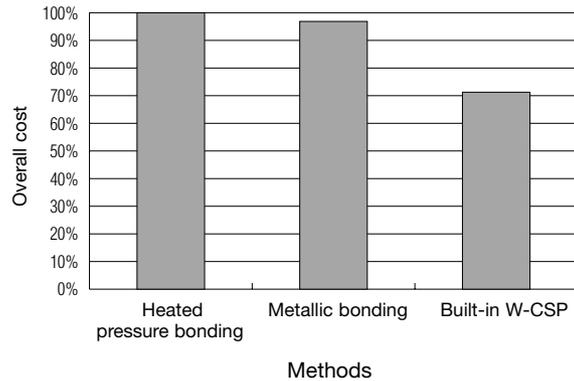
Fig. 3 Cost comparison of FC-type MCPs
