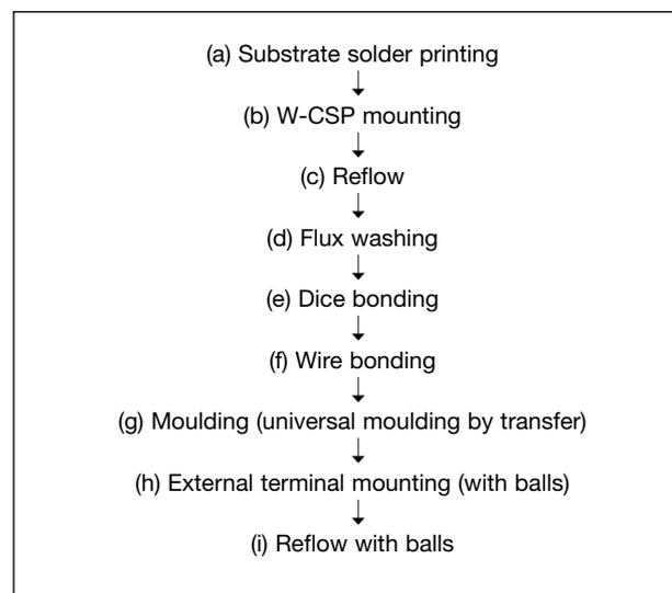
Fig. 4 Processing flow for MCP incorporating W-CSP
