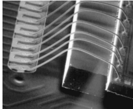
Fig. 6 WB results for second chip (wires extending beyond W-CSP)
