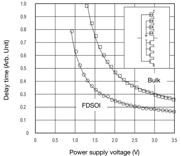
Fig. 3 Comparison of performance in 4NAND vertically integrated transistor
