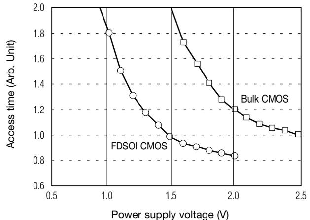
Fig. 1 Comparison of processor core performance
