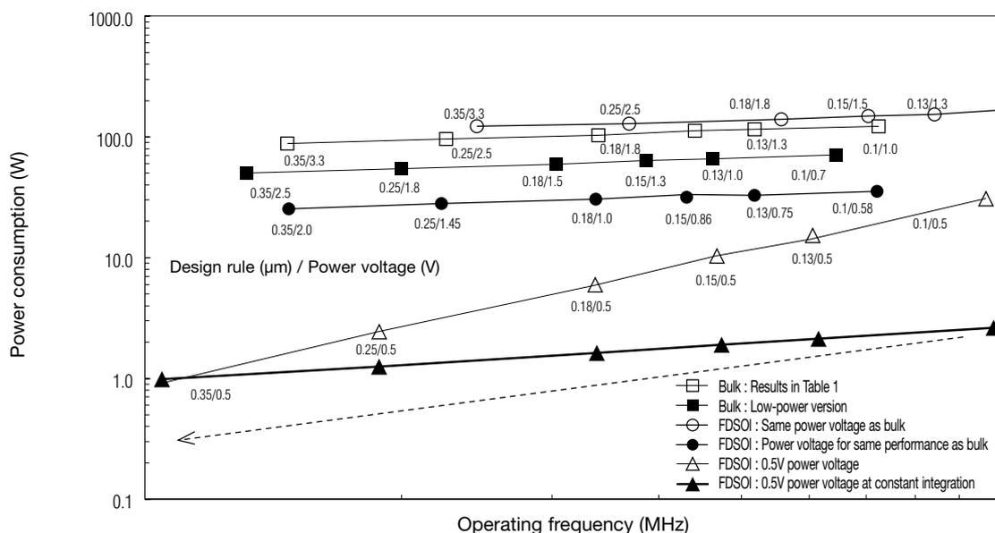
Fig. 4 Comparison of performance and power consumption
