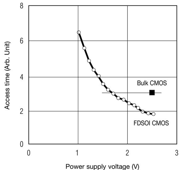
Fig. 2 Comparison of SRAM core performance
