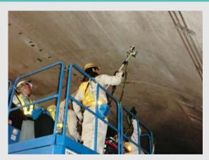
OKI has developed a tap-sound inspection device that can easily inspect for deformations in tunnels, such as spalling and detaching, using sound processing technologies, without reliance on veteran skilled labor.
