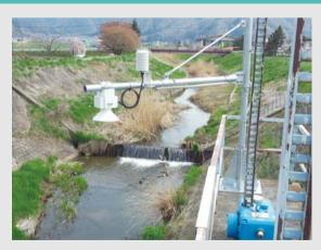
Our river monitoring system, which uses 920MHz band wireless multihop network technology, is fed various sensor data such as water levels and precipitation amounts from gauges set up at observations points along rivers via wireless transmission, enabling monitoring centers to collect data in real time and confirm changing river conditions.
