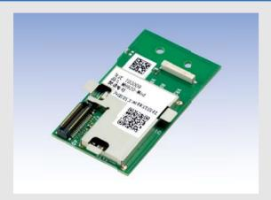
To go along with router types, which have conventionally performed the multi-hop relay function, we have launched coordinator types with wireless master-slave unit functions that aggregate for the purpose of connecting wireless multi-hop networks to online clouds, upper-layer data aggregation devices.
