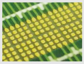
OKI Printed Circuits achieved a world-first breakthrough with massproduction technology for multilayer PCB to support 1,000-pin LSIs with a pin pitch of 0.35mm, harnessing its proprietary FiTT method, which fills a shortcoming in existing technologies, that draws on high-precision lamination and high-precision drilling technologies.
