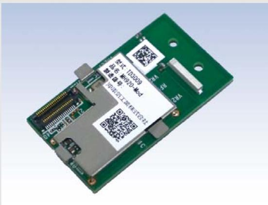
This telecommunication module adds a wireless function to sensors and measurement hardware, using our wireless 920MHz band multi-hop network technologies. This high-reliability module can easily be embedded into devices.
