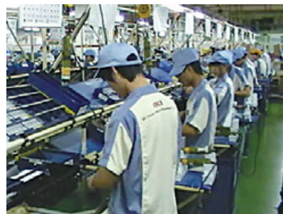
Assembly lines for banknote cassettes at our ATM manufacturing factory in Shenzhen, China.
