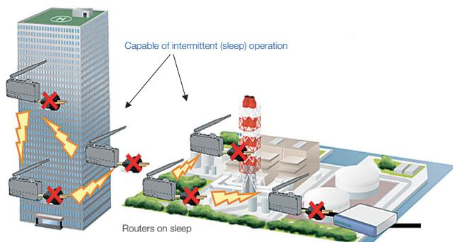
X : indicates AC mains connectors that are no longer required after battery operation is enabled
