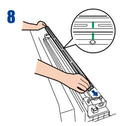
Install the new charger unit by aligning its | mark with the process cartridge's | mark.
