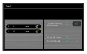
If waiting print jobs remain when turning the power off, the following message is displayed next time the power is turned on.
