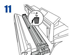
Rotate the knob at the center to remove it, and then dispose of it.
