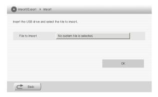
After the import process is finished, the Printer will restart when you exit the menu screen.
