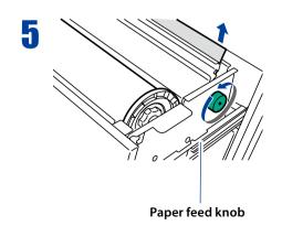
By rotating the paper feed knob, feed the roll paper so that a the top of the roll paper protrude from the printer by approximately 60 cm (23.63 inch).
