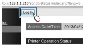
The authentication screen appears. Enter a login name and password. (For PIN code authentication, enter the PIN code in the login name field. Leave the password field blank.)
