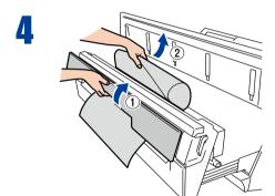
If the jammed paper cannot be pulled out from the Printer side, slightly pull the paper outlet cover to your side and lift up it. Then remove the jammed paper.
