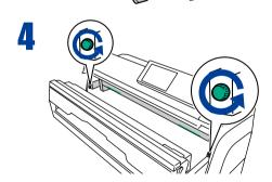
By rotating the right and left outerside knobs counterclockwise, release the process cartridge drawer's lock. Chapter **1**
