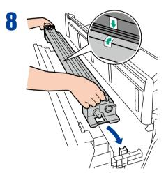
Remove the protective case of the process cartridge.
