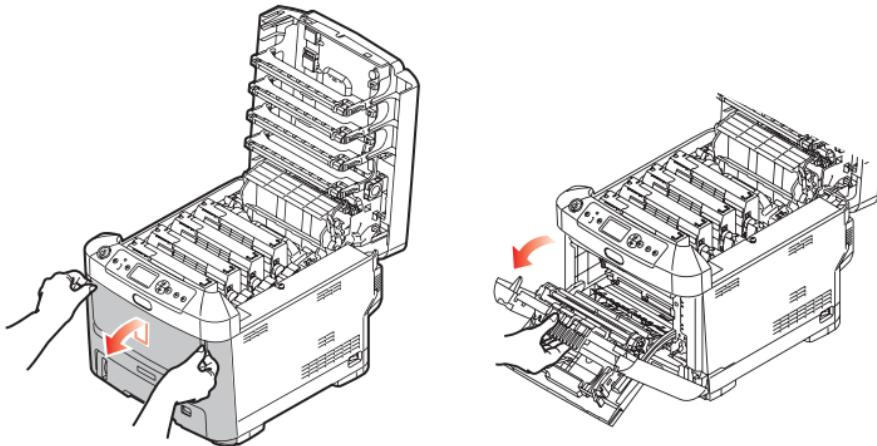
4. Loosen the screw (a) securing the right-hand side cover. Lift the edge of the side cover slightly and pull the cover away from the printer at the top. Lift the cover slightly to detach it from the printer. Place it safely to one side.
