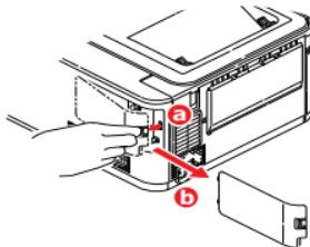
3. Turn the locking screw (a) counter-clockwise and remove the access cover (b). Put it aside in a safe place.
