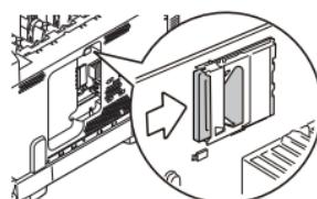
7. Locate the retaining clips at the bottom of the side cover into their rectangular holes near the bottom of the printer.
