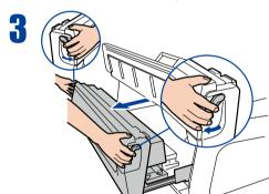
Lift the latch lever, and open the fuser unit drawer.
