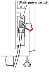
Turn on the main power switch on the bottom right when viewed from behind the Printer.
