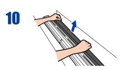
Remove the drum protective sheet.
