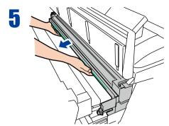
Pull out the process cartridge toward you by holding its green-indicated parts.
