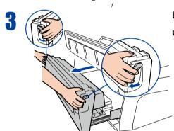
Lift the latch lever, and open the fuser unit drawer.
