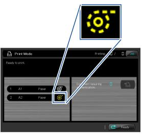
When the icon above is displayed, the Printer can output approximately 50 m (1968.50 inches) of printout. So get ready to replace the paper roll with a new one.
