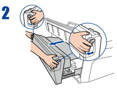
Lift the latch lever, and open the fuser unit drawer.
