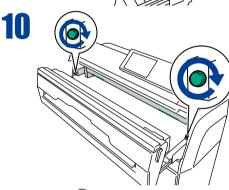
By rotating the outer-side knobs, fix the process cartridge.
