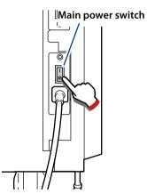
If the Printer will not be used for a long time, turn off the main power switch.
