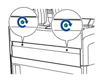
■ Removing a Paper Jam from the Roll Paper Drawer and the Front Door
