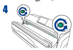
By rotating the right and left outer-side knobs counterclockwise, release the process cartridge drawer's lock.
