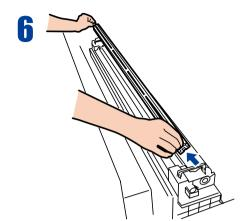
Pull the green handles to remove the charger unit.
