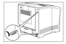
3. Slide the cover toward the rear of the printer and then downward to remove it.
