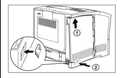
b. Slide the side cover towards the front of the printer to install it
