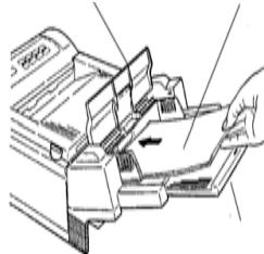
6. Load paper: Swing up paper feed cover and place paper (up to 100 sheets) or envelopes (up to 50) on tray. If paper is longer than 8-1/2", pull out support. Lower paper feed cover slowly and turn printer on.
