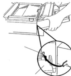
2. Install feeder: Insert hooks on Multi-Purpose Feeder completely into rectangular slots on printer.
