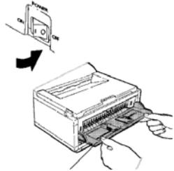
1. Prepare printer: Turn power off, then push in on manual feed tray and swing it down.
