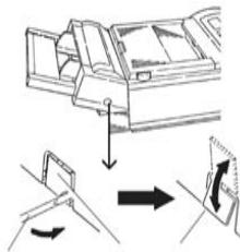
3. Remove feeder connector cover: Use flat-blade screwdriver to break side tabs on feeder connector cover. Then swing cover up and down until tabs break and cover snaps off.
