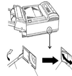
4. Remove printer connector cover: Use screwdriver to break side and top tabs, then swing cover back and forth until it snaps off. (This step not necessary if Second Paper Tray accessory is installed on printer.)
