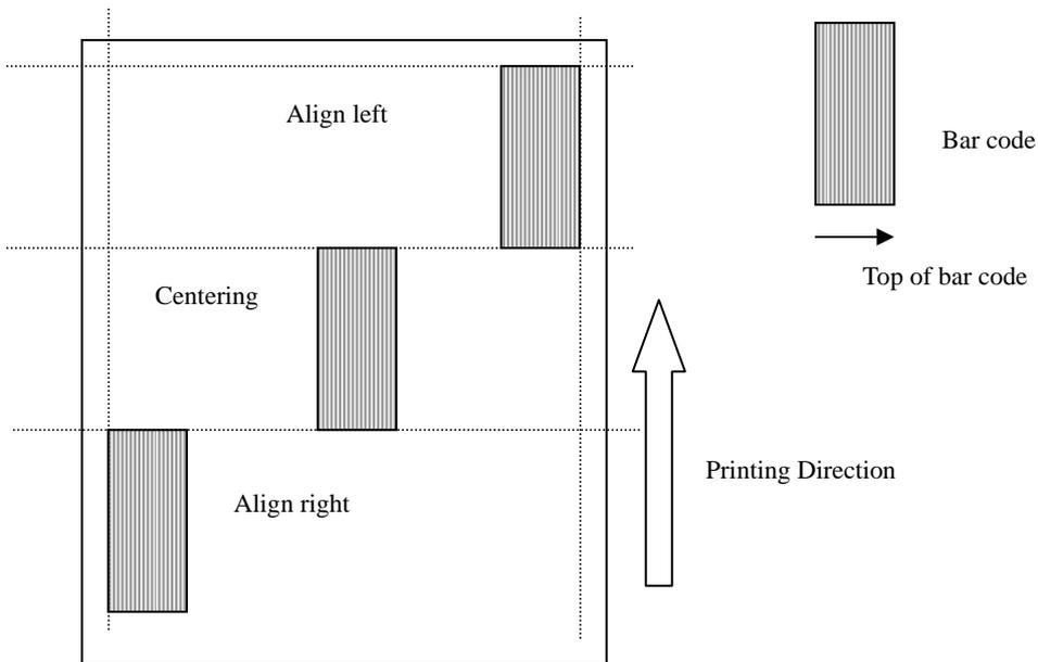
Printing positions are changed as follows by the *alignment* parameters in 90-degree-to-the-left orientation.
