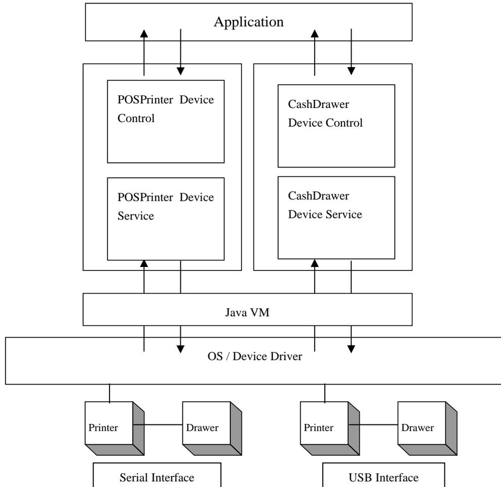
\*This JavaPOS Driver supports to control the Serial and USB Interface Printer and of at most two drawers each, connected to one printer.
