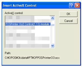
6. When OCX is inserted on the dialog box, select the control and right-click it. From the pop-up menu, select [Property]. Check the ID of the OCX. Clear the [Visible] and [Tab Stop] check boxes.
