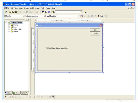
5. On the dialog box, right-click to display the pop-up menu, and select [Insert ActiveX Control]. When the dialog box is displayed, select [POSPrinter OLE Control (1.13) module] and select [OK].
