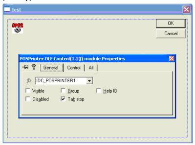
7. Close [Property], repeat the step 6 and select [ClassWizard]. Select the [Member Variable] tab, select the control ID checked in the step 6, and press [Add Variable].
