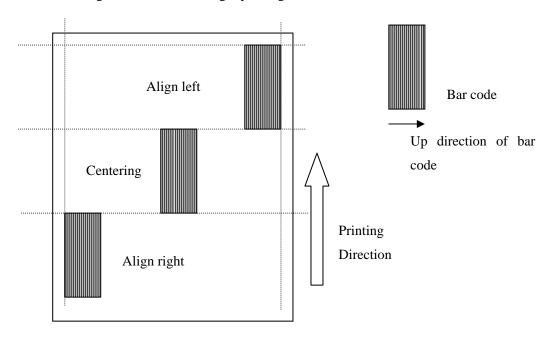
Printing-position-change by *Alignment* assignment, at the time of 90-degree-rotation-to-the-left printing.
